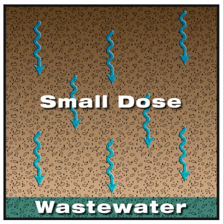
Small dose spreads over the bottom of the trench, allowing the wastewater to infiltrate into the soil before the next dose is applied #16
